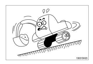
Avoid parking and stopping on a slope. Lower the bucket to the ground and block the track when parking.
